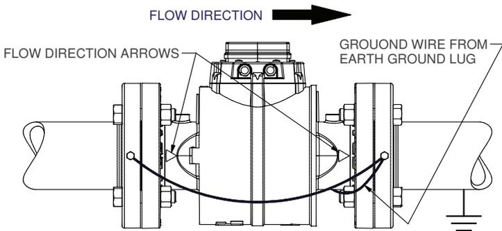
TYPICAL INSTALLATION IN STEEL CONDUCTIVE PIPE
