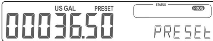
Fig. 3: Example display information during programming preset value.
